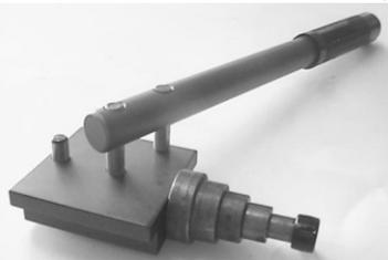
1. Secure bender to workbench or clamp in a vise.
