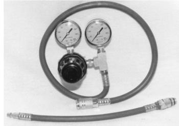
Unit is complete with three-foot hose, quick-disconnect fittings, 14 mm & 18 mm adapters with two foot whip.
